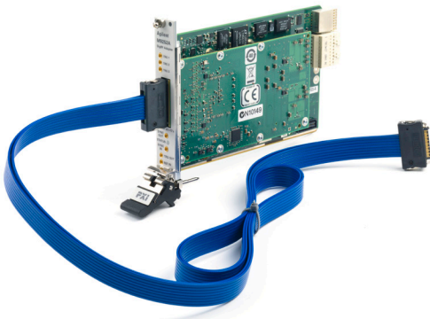
M9252A DigRF host adapter module and M9255A DUT cable
